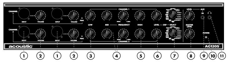
The AG120S Acoustic Performance system is designed for up to four inputs, which can be any combination of microphones and instruments. One suggested operation of the AG120S would be to use Channel 1 for vocal microphones, and Channel 2 for instruments. Its EQ and effects can be tailored for each channel independently, while the Stereo Aux Input (see #9) allows for true stereo playback of your MP3 device.
